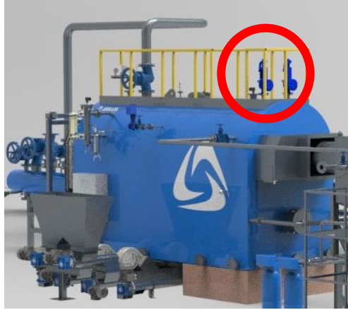
Figure Ap. 4.7 Safety Valves
