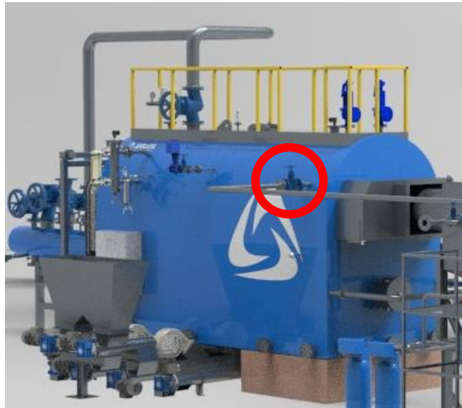
Figure Ap. 4.6.1 Boiler Water Inlet Valve & Check Valve
