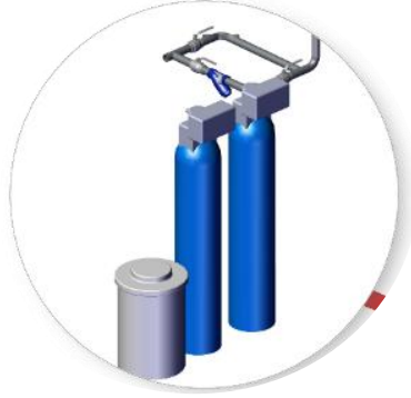
Figure Ap. 4.17 Water Softener
