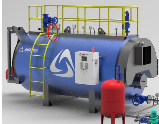
Figure Ap. 4.8 Temperature Switch
